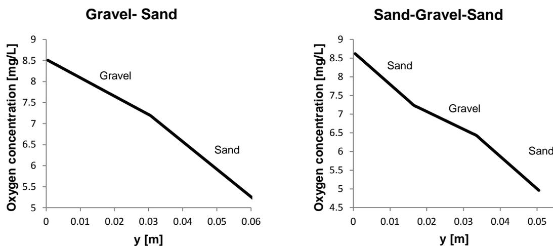
Figure 6: Longitudinal profile of oxygen concentration through the centre of the microcosms.
