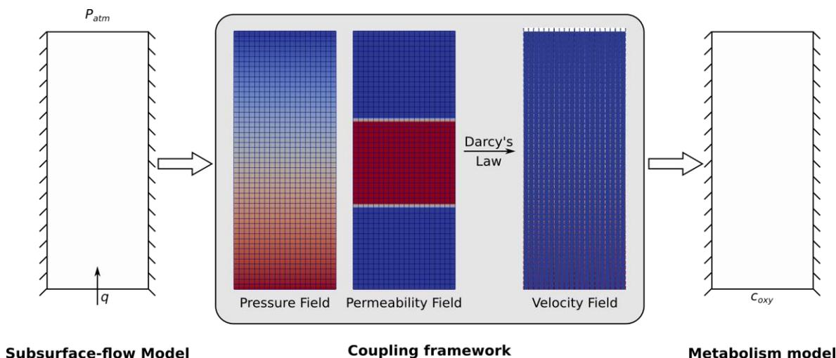
Figure 2: Schematic diagram of the coupled subsurface-flow and Hz metabolism model with the software framework for coupling models acting as the coupling broker.
