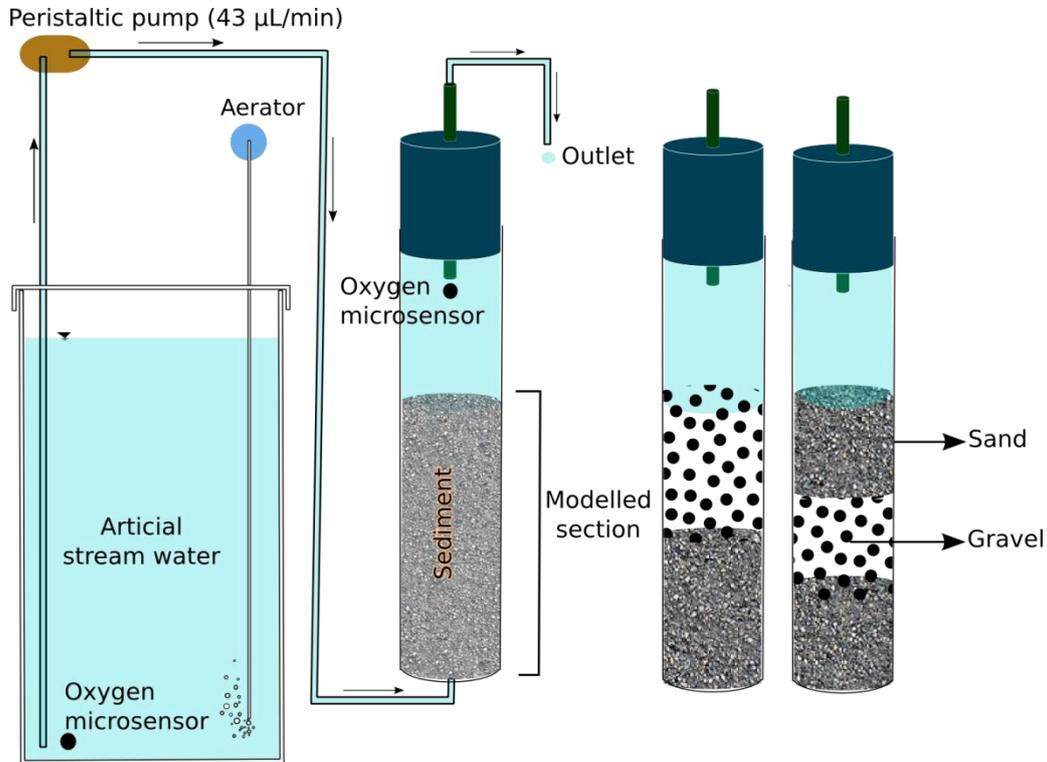
*Figure 1: Schematic representation of the experimental set-up: example with one percolating microcosm filled with uniform sediment, and the different combinations of gravel and sand measured (uniform, 2- and 3-layers perpendicular to flow direction).*
