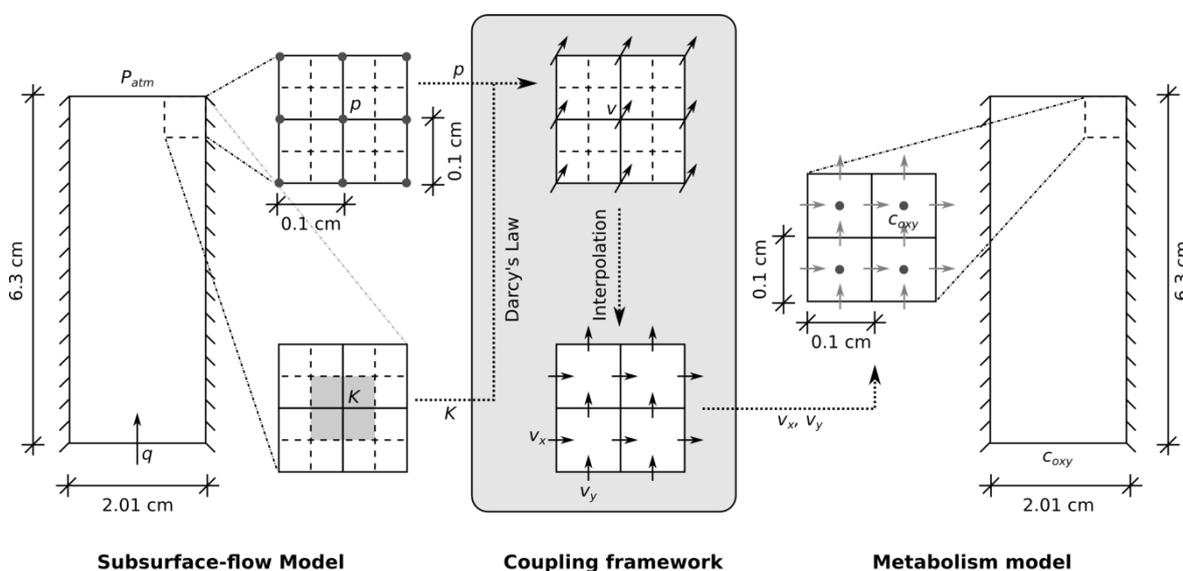
Figure 3: Dimensions and space discretisation of the subsurface-flow and Hz metabolism model.
