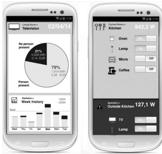
Figure 1 Using room-context information to enrich eco-feedback visualization (left) and to adapt home control interfaces (right)
